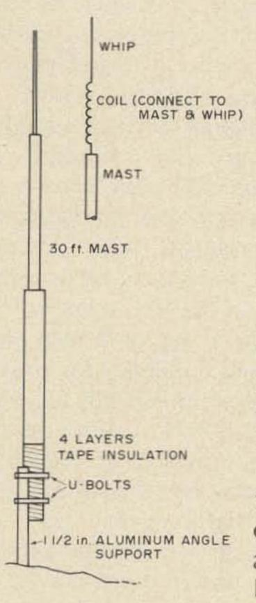
thirty-foot vertical, top-loaded and La using as good a ground as possible, can produce good results on 160. The antenna described here was designed for field day and portable operation, but may be made a permanent installation. It makes use of readily available materials and is inexpensive to build and easy to tune up.
