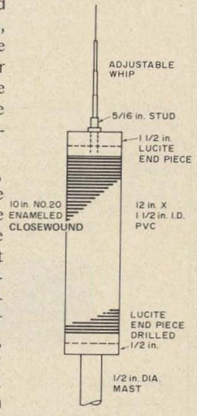
string for guys, but if a permanent installation is to be made, wire guys and suitable insulators should be used. Four layers of scotch electrical tape are wound over the bottom of the mast as an insulator, although a better insulator might be made by using a section of old bicycle innertube slipped over the end of the mast.
